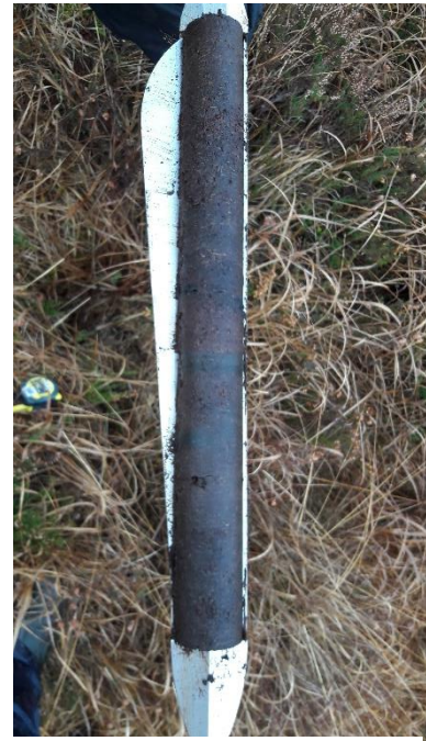
Peat coring with a Russian auger to determine bulk density values Photo: David Wilson.
