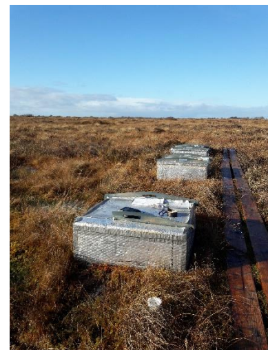
Dark chambers used to measure CH 4 fluxes at Moyarwood, Co. Galway. Photo: David Wilson.
