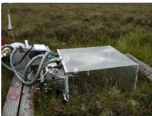
Transparent chamber used to measure CO 2 fluxes at Clara, Co. Offaly. Photo: David Wilson.
