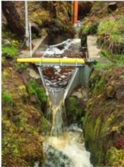
V-notched weir and instrumentation to measure dissolved organic carbon (DOC). Photo: Mark O'Connor.
